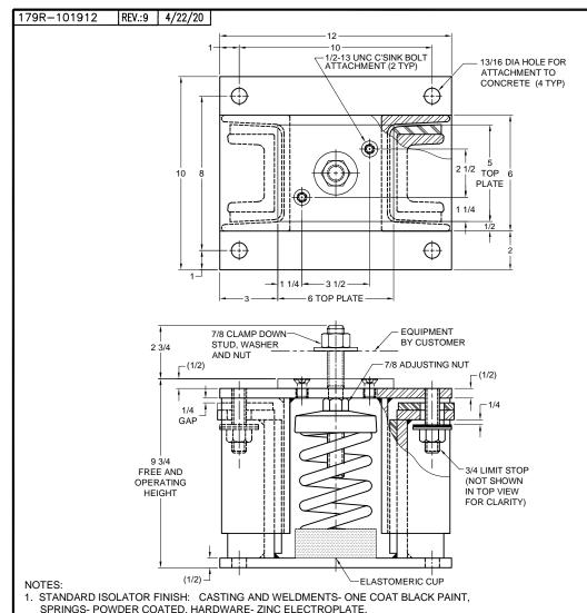
3. STATIC LOAD RATINGS ON SHEET 2 OF 2 ARE FOR GUIDANCE ONLY. VALUES ARE BASED ON TESTS OR CALCULATIONS
